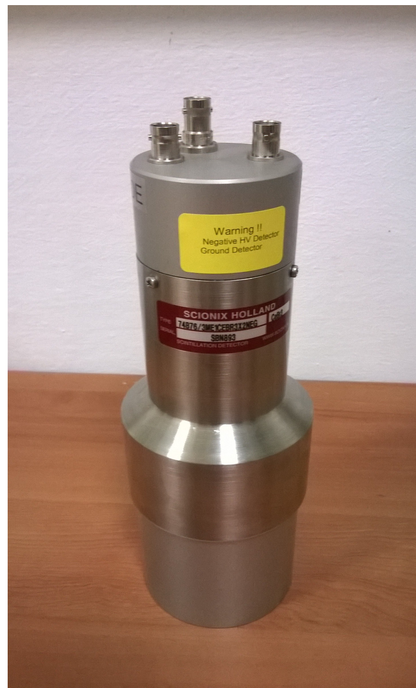
Fig. 1 CeBr 3 scintillator (3"x3") coupled to R6233 PMT.
