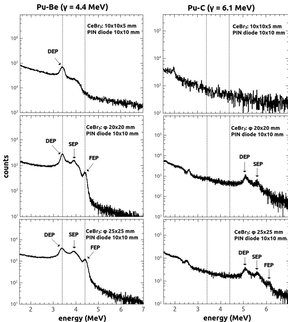
**Fig. 1.** Comparison of gamma spectra from PuBe and PuC sources for CeBr<sub>3</sub> scintillators: 10×10×5 mm, Ø20×20 mm, Ø25×25 mm, coupled to 10×10 mm PiN-diode. Dashed vertical lines are limiting the GCU region-of-interest.
