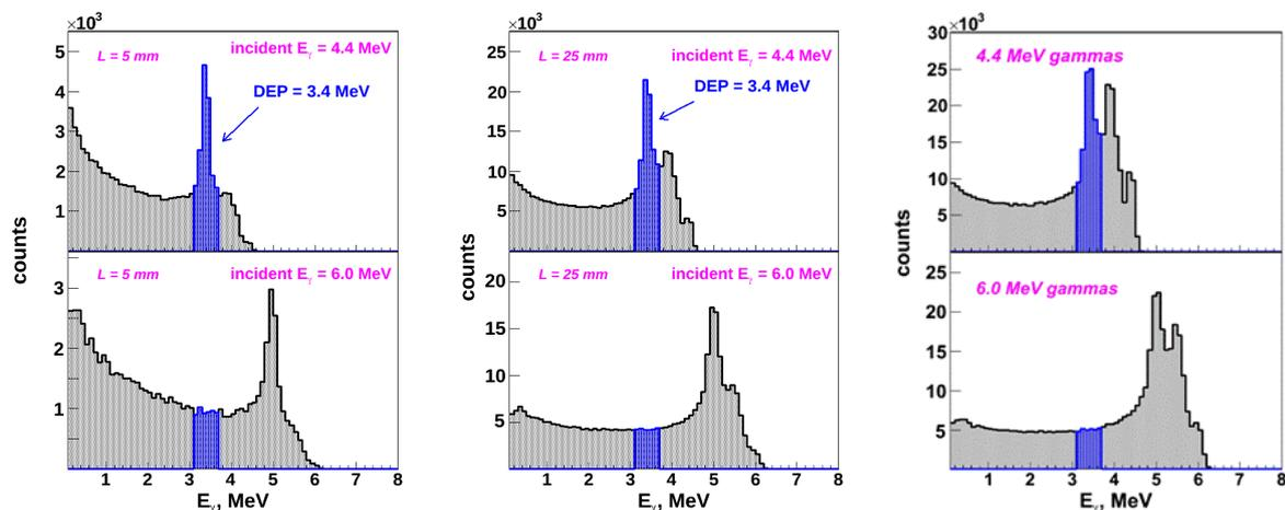
**Fig. 2.** In the left part, spectra obtained for a scintillator with a diameter of 20 mm and a thickness of 5 mm irradiated by gammas with energies of 4.4 (upper) and 6.0 MeV (lower) are compared. In the central part, such a comparison is shown for a scintillator with a diameter of 20 mm and thickness of 25 mm. In the right part, the scintillator has dimensions of 35×35 mm.
