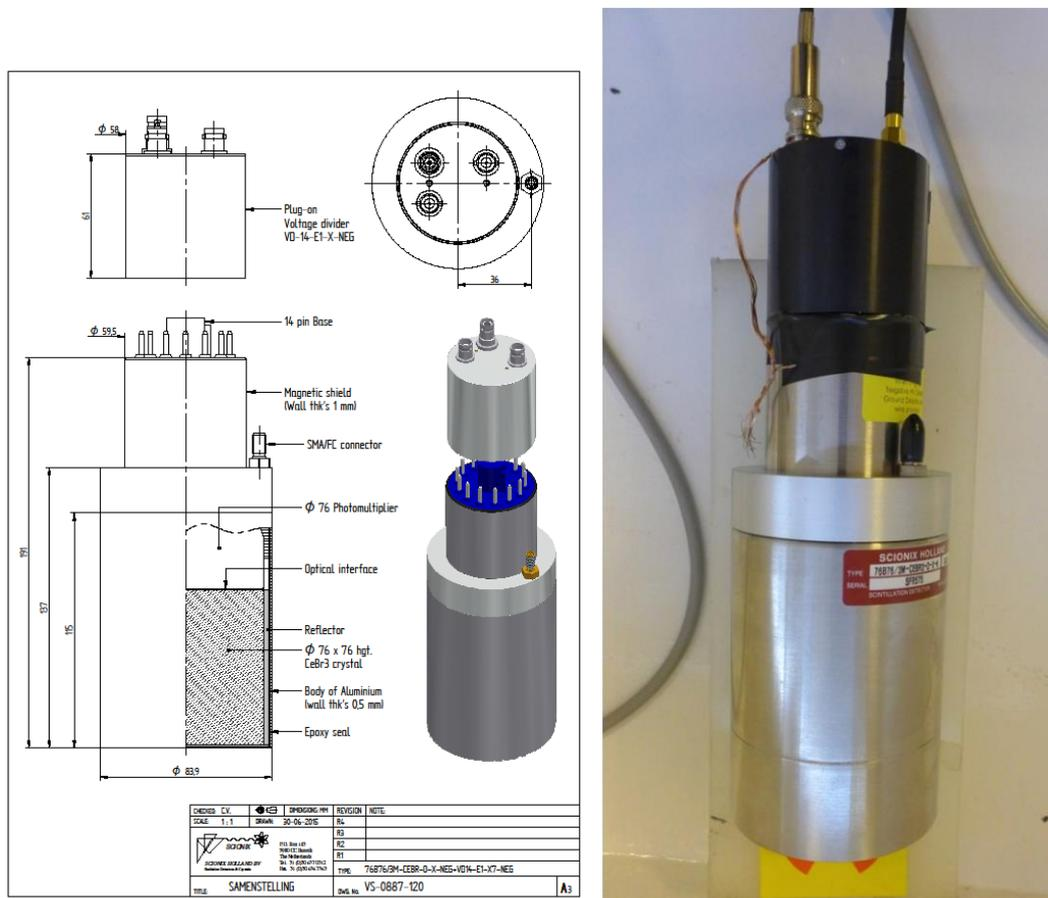
**Fig. 1.** 3''x3'' CeBr<sub>3</sub> from Scionix: a technical drawing and a photo.
