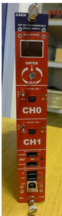
**Fig. 2.** CAEN N1470A high voltage power supply.
