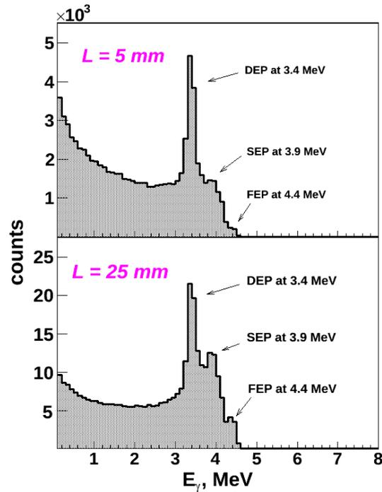
Fig. 1. Monte Carlo simulated gamma-ray spectra for a LaBr<sub>3</sub> scintillator obtained for 4.4 MeV gamma rays incident on a crystal with a thickness of 5 mm (upper) and 25 mm (lower).
