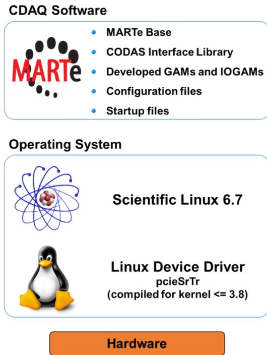
Fig. 3 - Software Architecture
