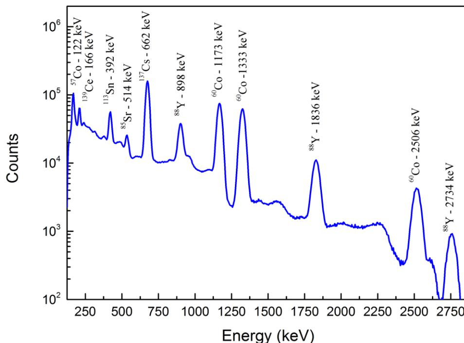
**Fig. 1.** Spectrum recorded with a 3"×3" CeBr<sub>3</sub> scintillator measured with a mixed source No. AG-5430 and registered with the CAEN digitizer.
