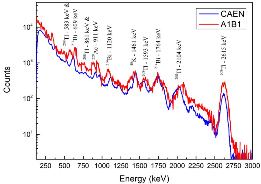
**Fig. 4.** Comparison background spectra measured with two data acquisition systems: CAEN and TRP-400 (PHA post processing method – A1B1).
