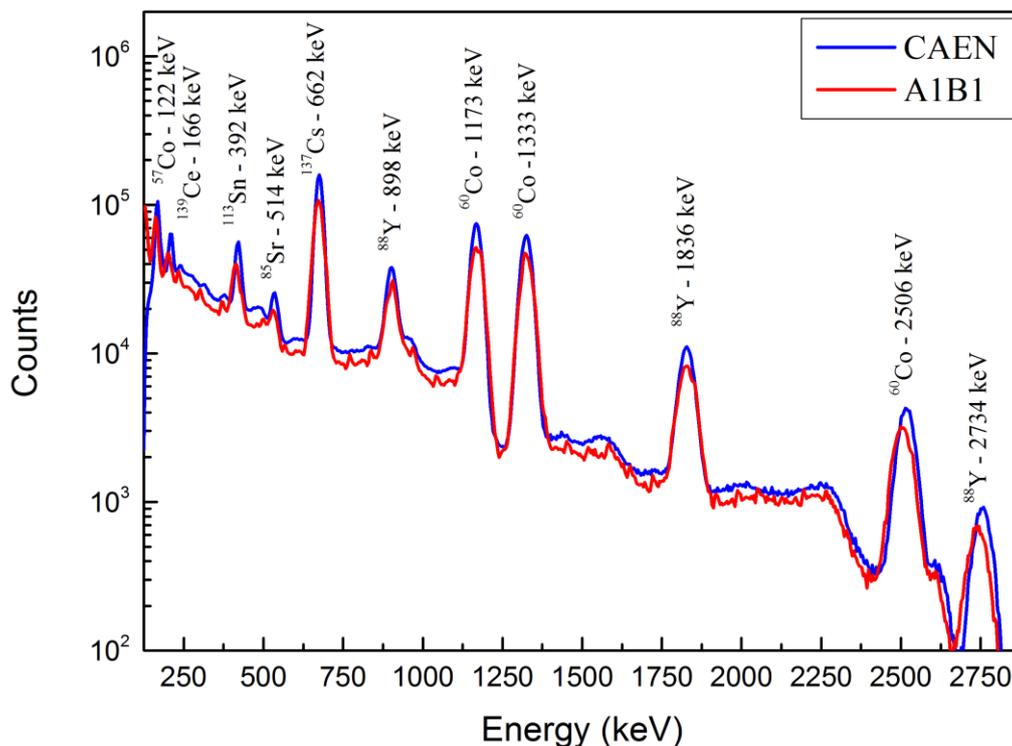
**Fig. 2.** Comparison of spectra registered with the 3"×3" CeBr<sub>3</sub> scintillator and both CAEN and TRP-400 (using a PHA post-processing algorithm (A1B1)), data acquisition systems. Measurements were performed with a mixed source in the energy range between 122 and 2734 keV.
