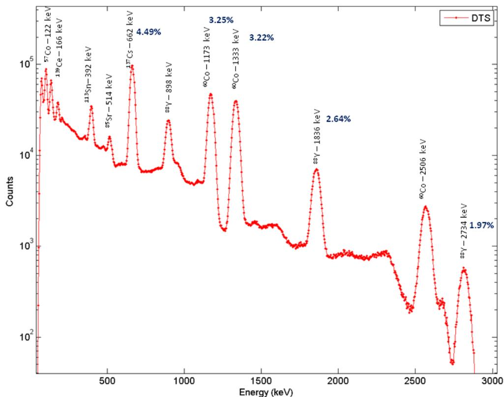
Fig. 5. Spectra obtained with DTS post-processing method, from data acquired with TRP-400 in presence of the mixed source No. AG-5430. Measurements were performed with a mixed source in the energy range between 122 and 2734 keV. Event rate of 2 kHz.
