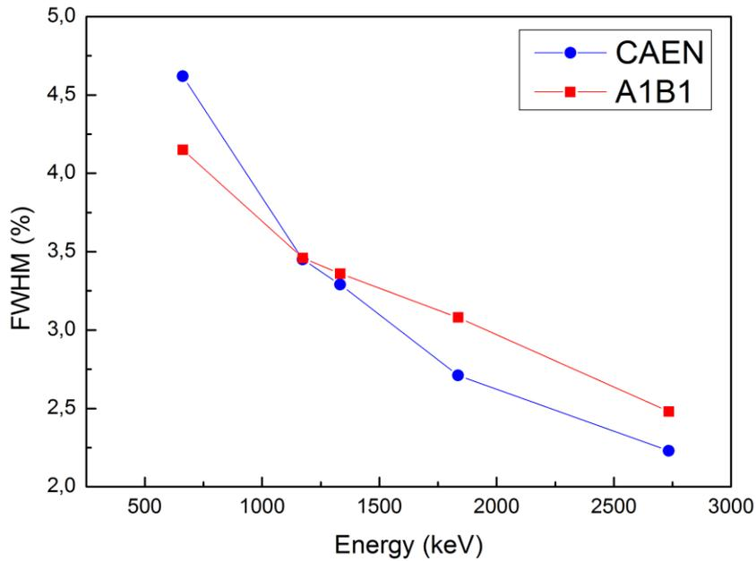
**Fig. 3.** Comparison of measured values of FWHM obtained with both data acquisition systems: CAEN and TRP-400.
