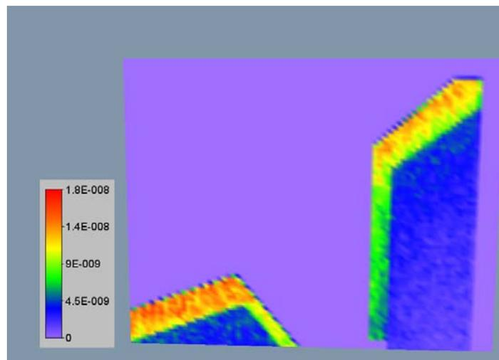
Fig. 7: Graphical presentation of the density of the (n, n' 1<sup>st</sup> excited state)  $\gamma$  reaction in the divertor. Presented as the number of reactions per cm<sup>3</sup> of material.
