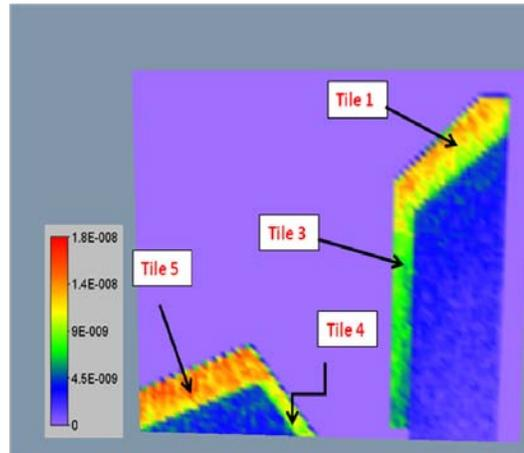
Figure 8.8: Density of prompt gamma emission in the CFC divertor (number of reactions per  $\text{cm}^3$  of material).
