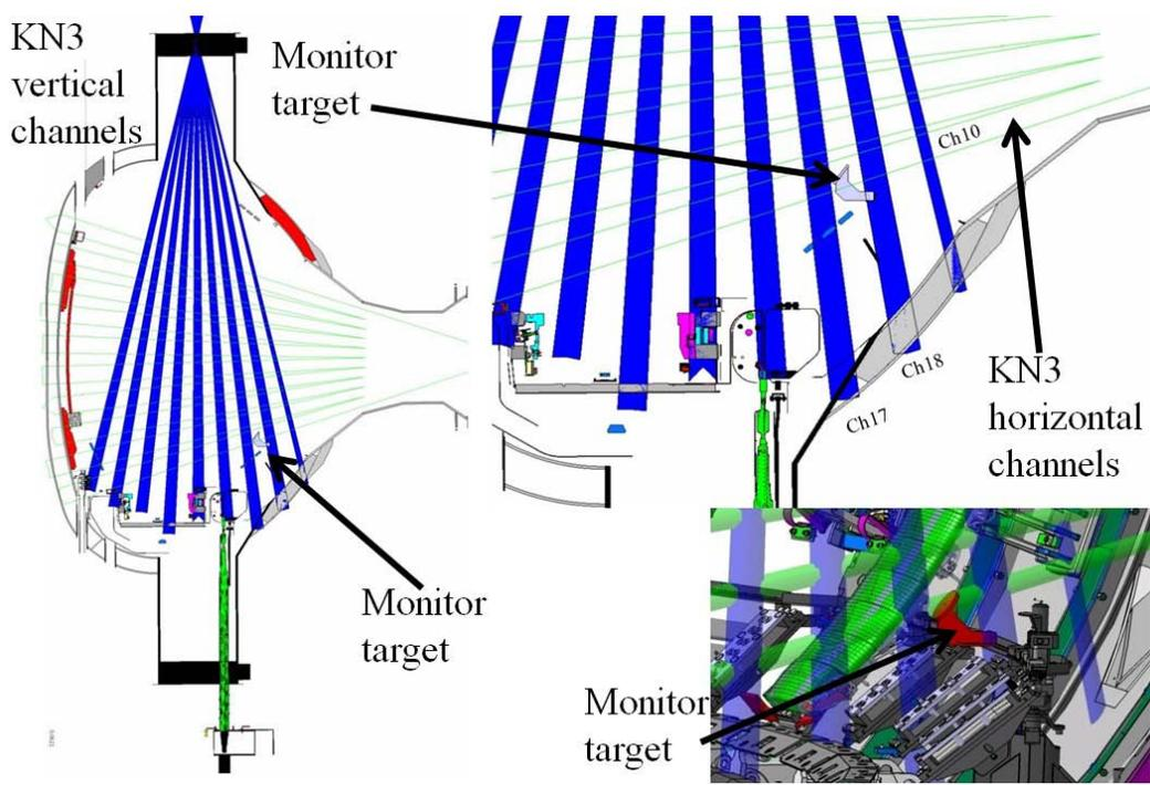
Figure 4.1: LAM target location on the KN3 channel 10
