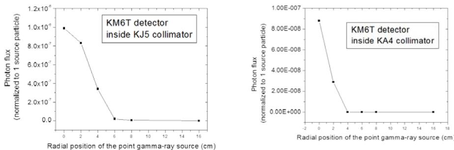
Figure 8.9: Gamma-ray source profiles: inside the KJ5 collimator (LHS), and inside the KA4 collimator (RHS)
