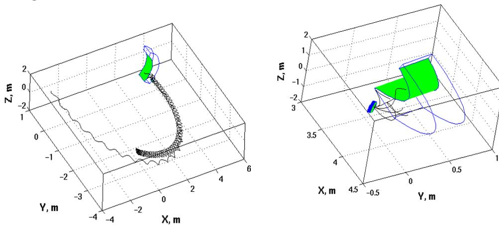
Fig.2. Example of backward-in-time trajectory calculations starting from one point on the LRM target (left) and a subset of the trajectories hitting the wide poloidal limiter (right). The target pellet is blue-colored.
