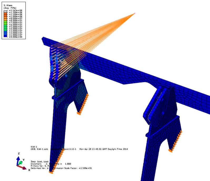
Figure 7 FE Model showing coupling from a remote point to represent a nominal halo load of 1 kN (in z). FE Ref: KA4-1b
