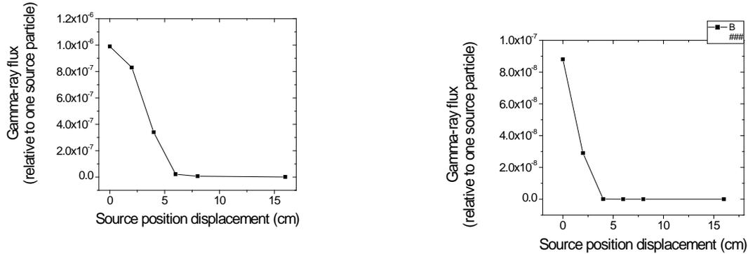
Figure 5: The dependence of the photon flux on the source position for the detectors located on the KA4 diagnostics axis of symmetry in case of KJ5 (left) and KA4 (right) radiation shields.
