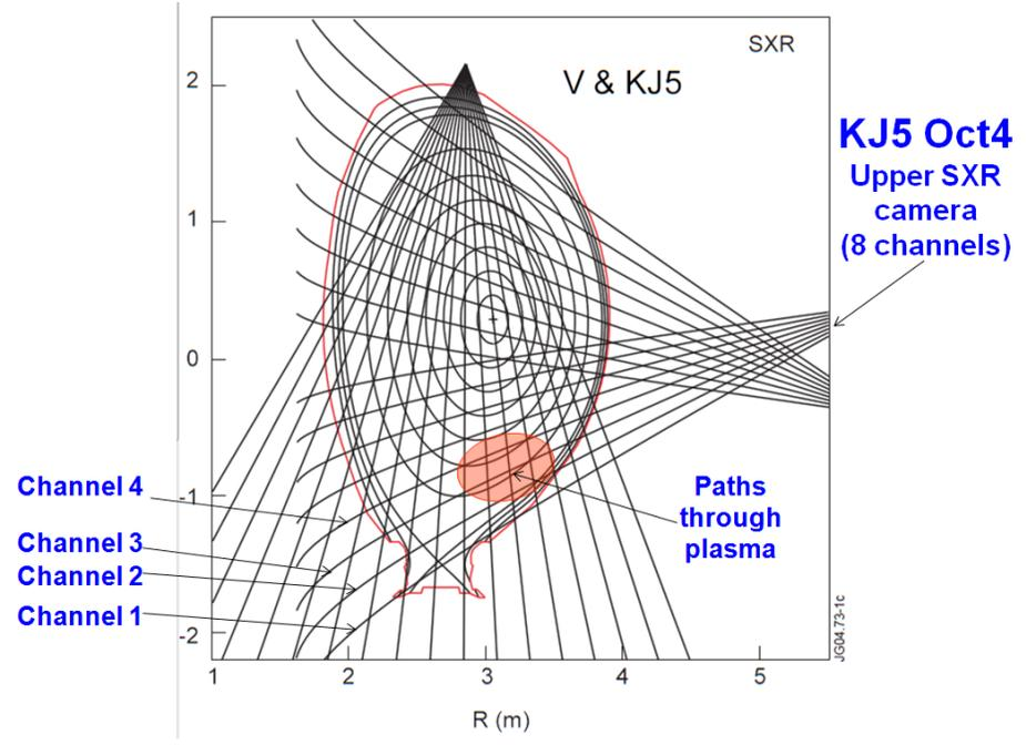
Figure 3.3: KJ5 upper Soft X-ray camera
