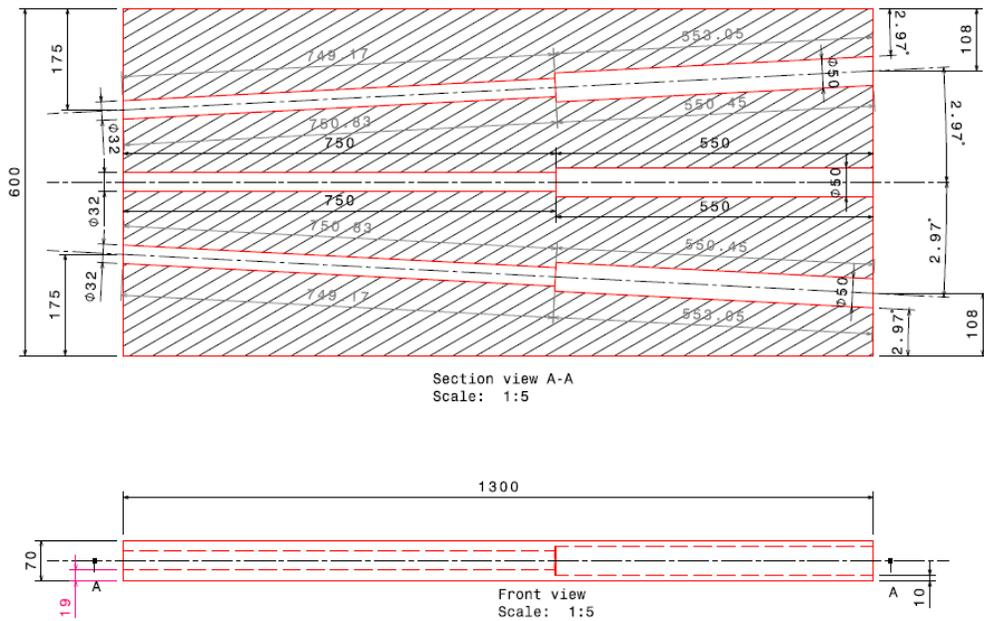
Figure 5.5: KA4 collimator
