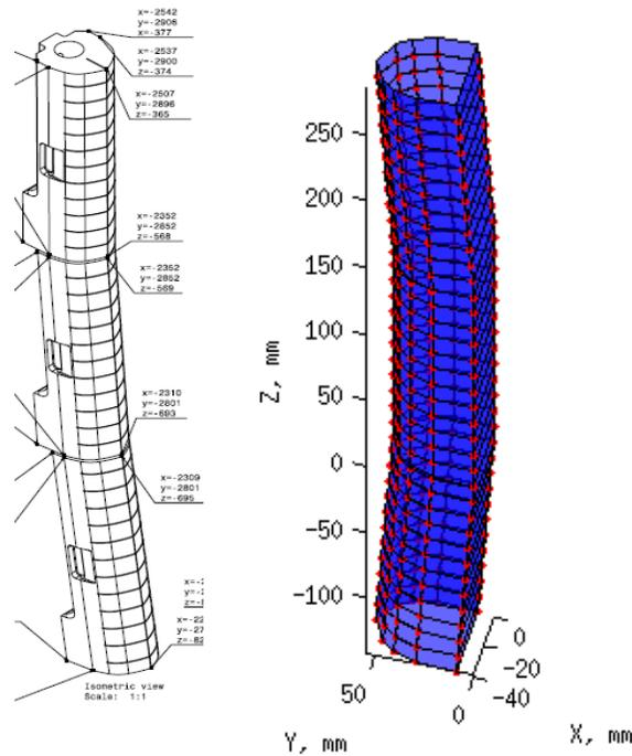
Figure 8.4: CATIA drawing of the Be TAE antenna protection tile (left) and the numerical model of the tile (right) with the starting points for test trajectories marked in red
