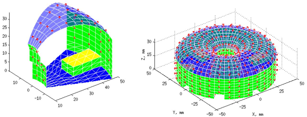
Fig.6. Numerical model of a Be mushroom tile (1/8 element on the left) with the starting points of the test trajectories marked in red.
