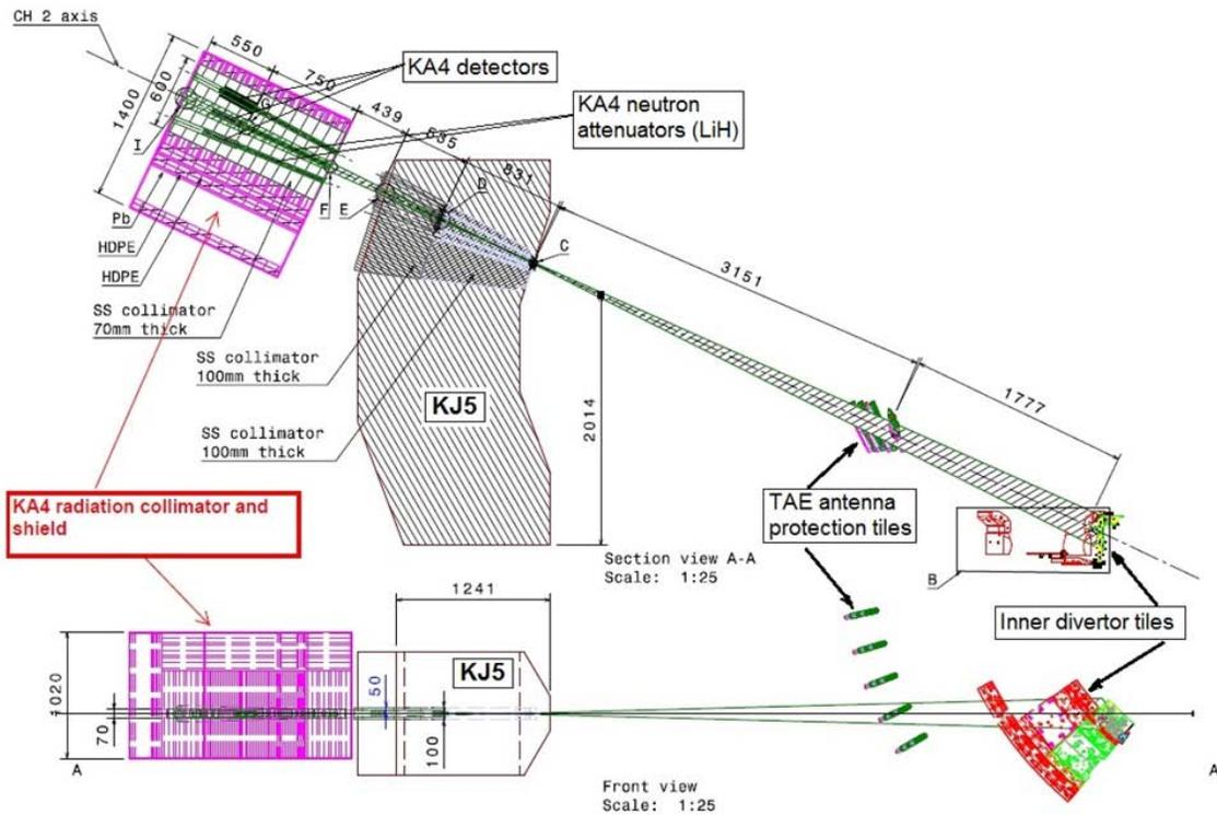
Figure 5.1: KA4 radiation system. Top: vertical cross-section containing channel #2, 3, and 4. Bottom: “horizontal” cross-section through channel #2.
