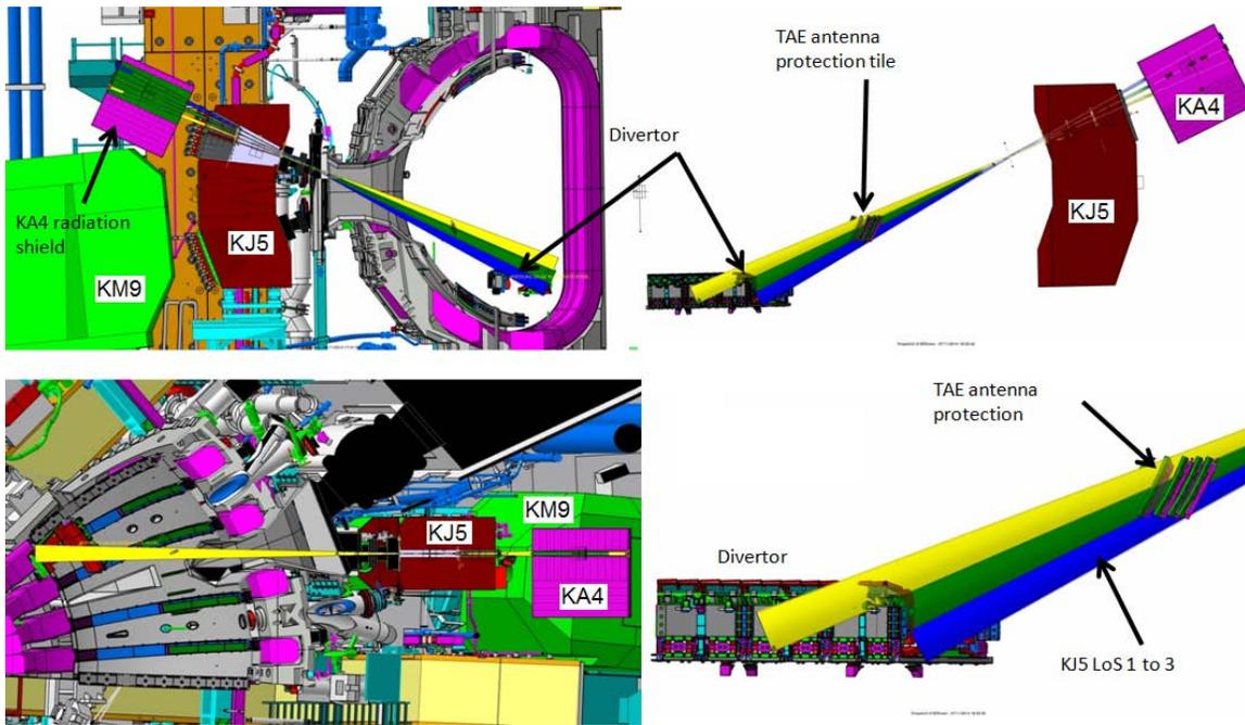
Figure 5.3: KA4 radiation collimator and shield showing its position with respect to the adjacent JET diagnostics: KJ5 soft X-ray camera and KM9 magnetic proton recoil spectrometer. The FoV's for channels #1, 2, and 3 are also shown crossing the TEA antenna protection tiles and ending on the inner divertor tiles.
