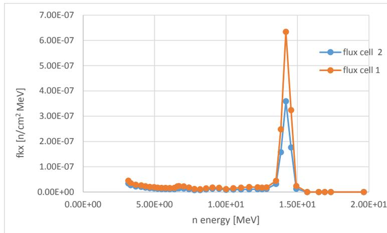
The corresponding total fluences above 4 MeV are  $6.47E-07$  n/cm<sup>2</sup> for cell 1 and  $3.96E-07$  n/cm<sup>2</sup> for cell 2 per source neutron in the plasma.
