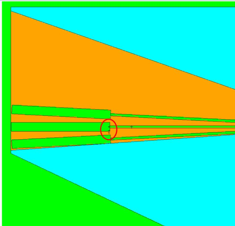
Figure 3 – MNCP geometry detail showing the location of the virtual detectors inside the KJ5 radiation shield (circled in red)
