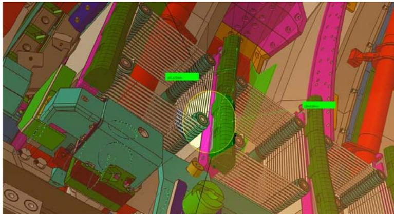
Figure 3.7: KA4 target: TAE tile surface in the channel 2 Field-of-View
