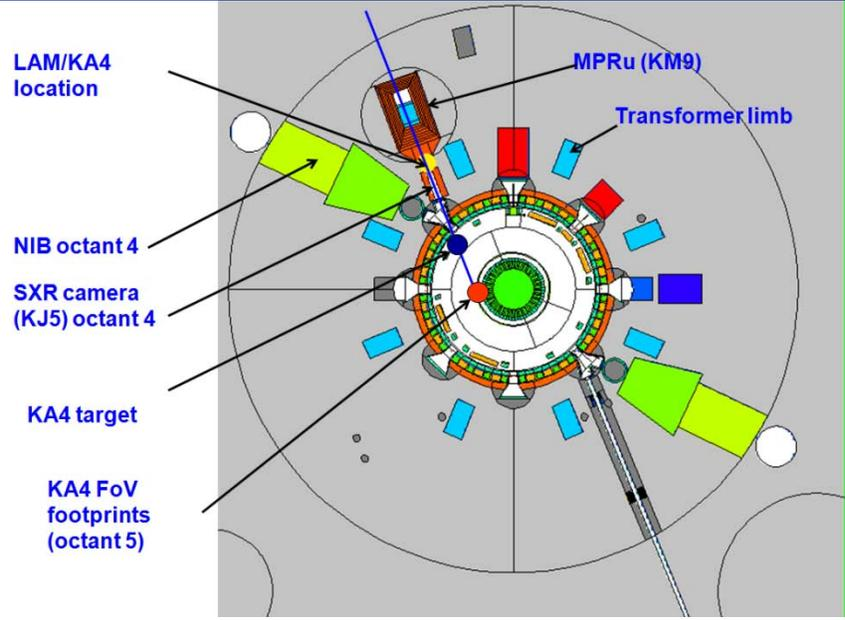
Figure 3.2: Location of the LAM/KA4 diagnostics on the KJ5 soft X-ray camera in octant 4
