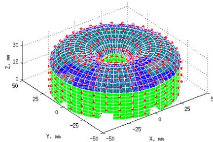
Figure 8.1: Numerical model of a Be mushroom tile with the starting points of the test trajectories marked in red
