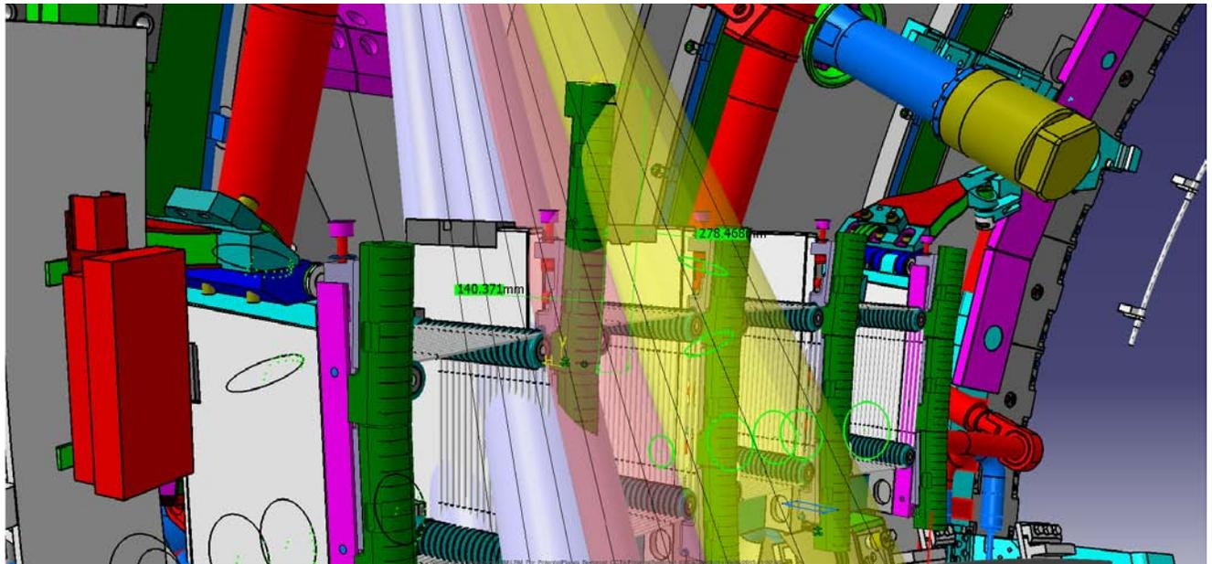
Figure 1 – Extended upper beryllium tile (middle) of the TAE limiter. Extended carrier is not shown.
