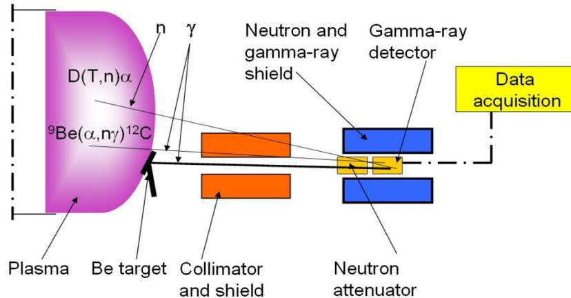
Figure 2.1: schematic diagram for the LAM principle
