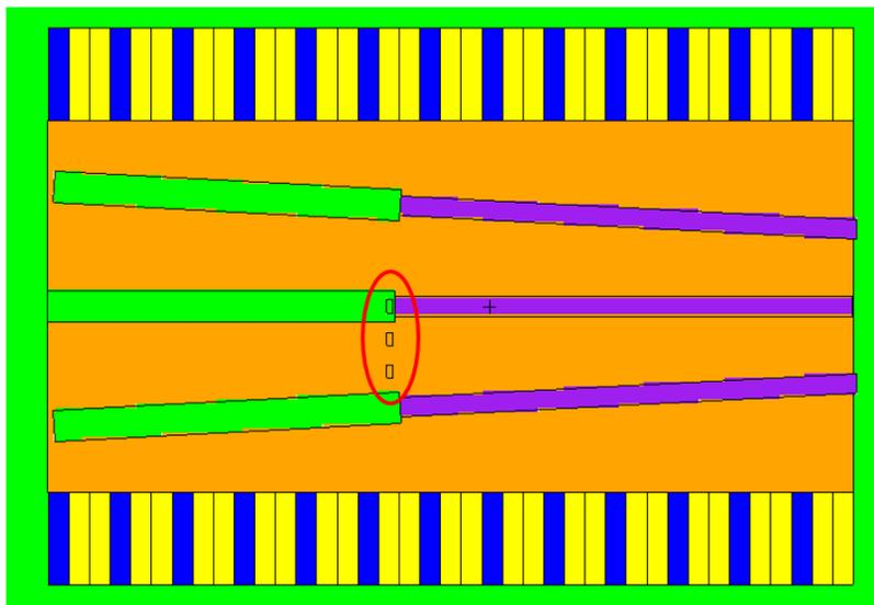
Figure 4 – MNCP geometry detail showing the location of the virtual detectors inside the KA4 radiation shield (circled in red)
