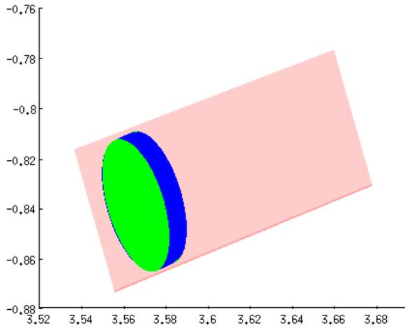
Figure 8.2: Optimal position and orientation of a disc-type LAM target (green and blue) in channel #10 FoV (pink).
