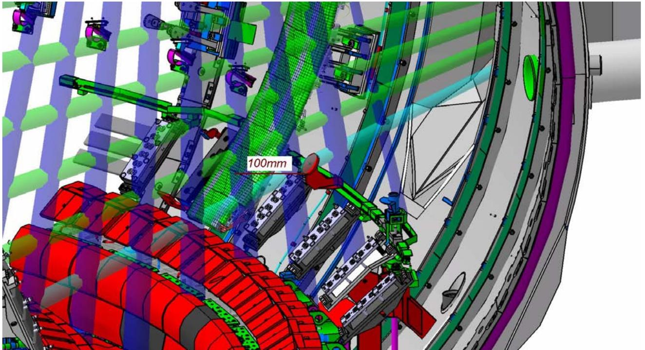
Figure 1. KA4 Lost Alpha Particle Target in Sector 1C
