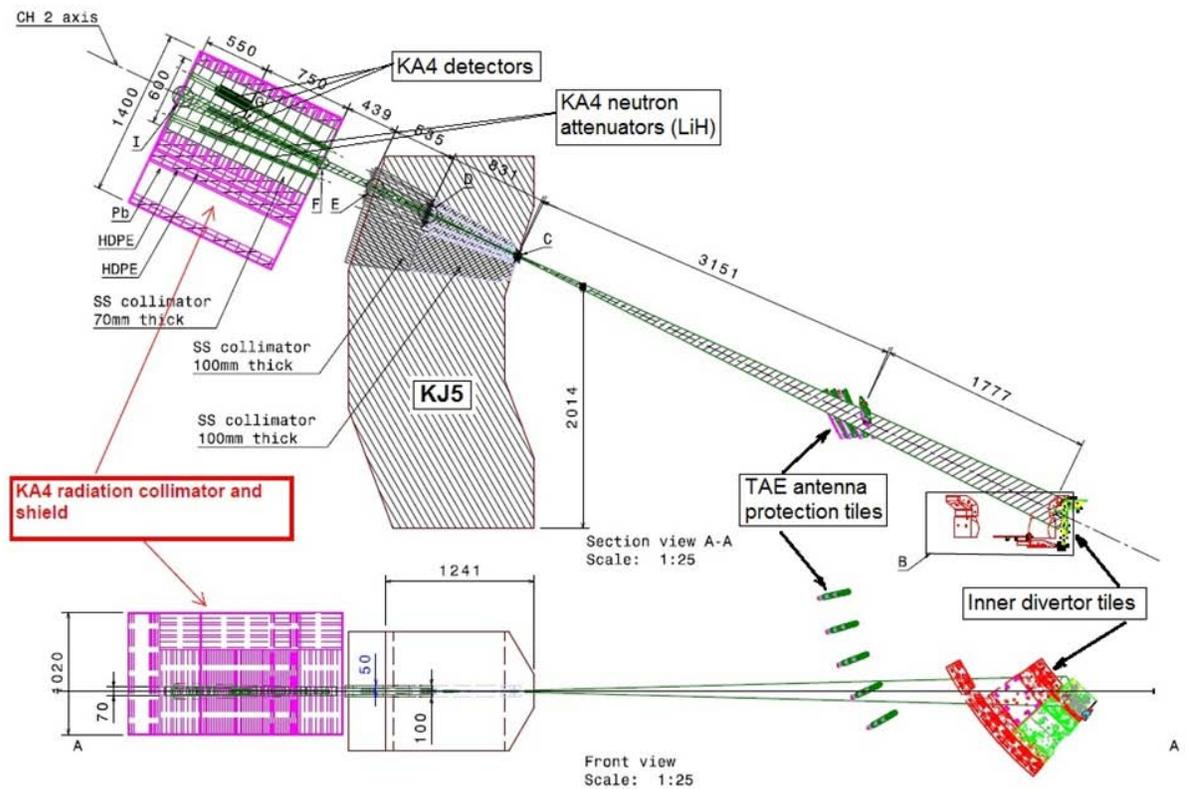
Figure 1: Overall view of the LAM/KA4 radiation system
