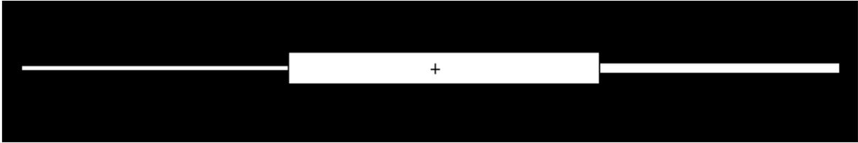
Fig. 8: Simple MCNP model of the collimator line of sight; presented is only the collimator and not the origin of the divertor gammas, located 5m from the collimator to the left.
