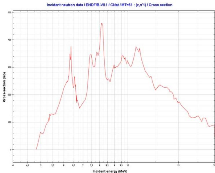
Fig. 4: Cross section for neutrons in  $C^{nat}$  for 4.439 MeV gamma production.
