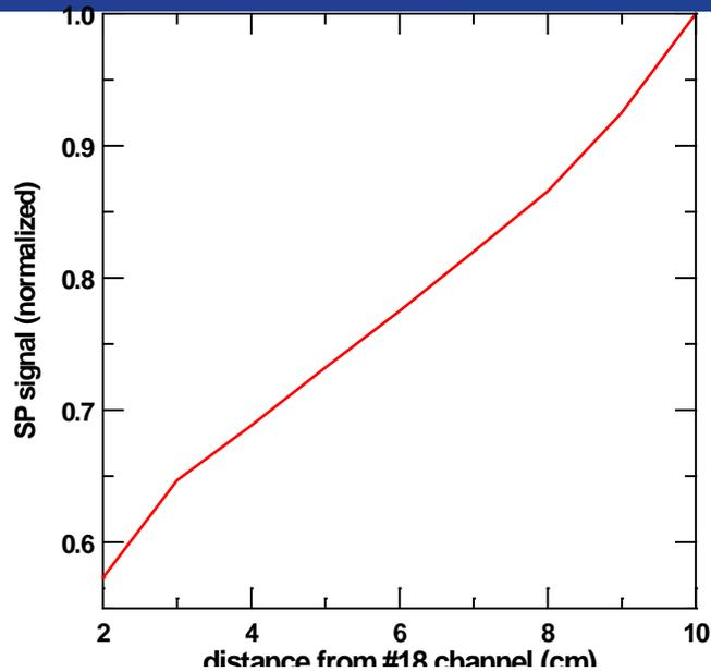
Fig.5. Dependence of the relative signal intensity when the LRM target is moved from a position 2cm apart from the channel #18 Line of Sight towards a 10 cm distance (close to channel #17). Normalization is to the maximum value.
