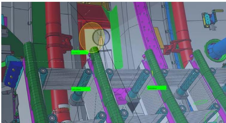
Figure 3.9: KA4 target: TAE tile surface in the channel 4 Field-of-View
