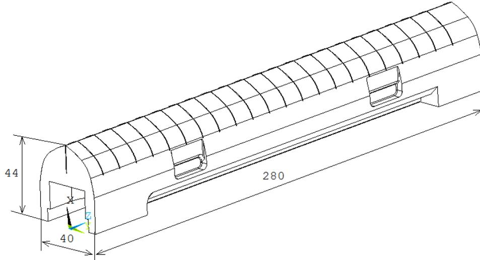
Figure 2 – Longer tile overall dimensions.
