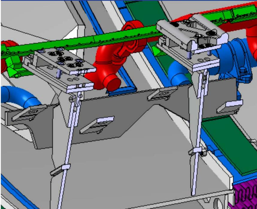
Figure 6 Sector 1C showing lower outer saddle coils where probe may be supported.
