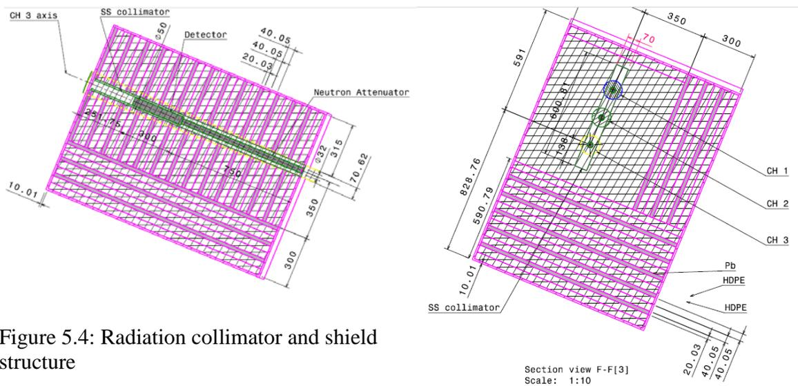
Figure 5.4: Radiation collimator and shield structure
