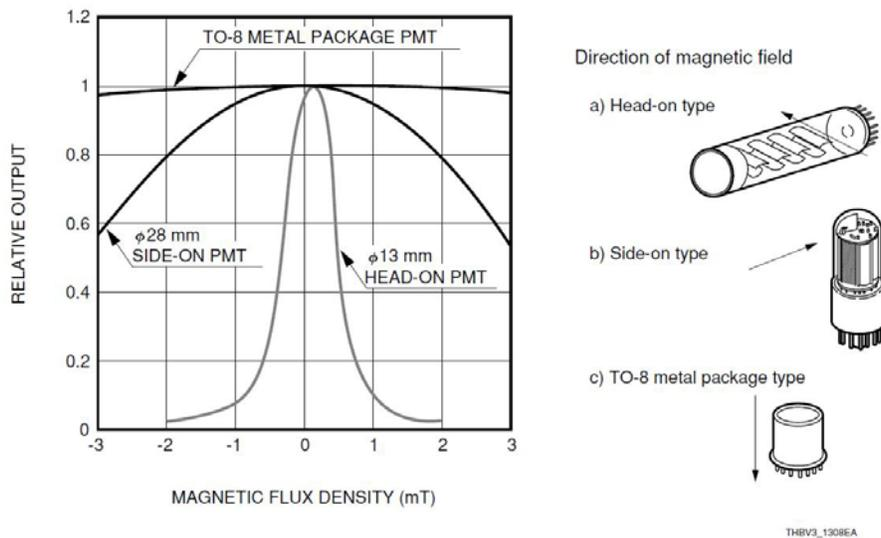
Figure 1: Magnetic characteristics of typical photomultiplier tubes
