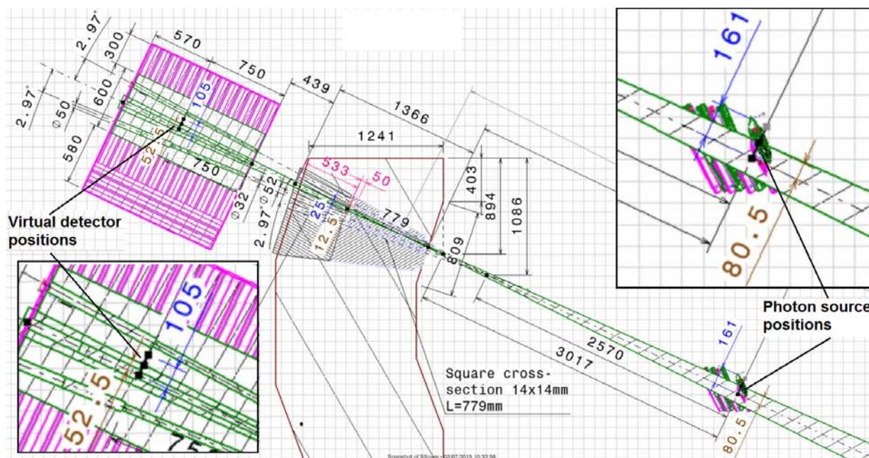
Figure 2: Positions of the photon source and virtual detector. The inserts are zoomed-in views of the target region (photon source) and detector region, with the detector inside the KA4 radiation collimator and shield.
