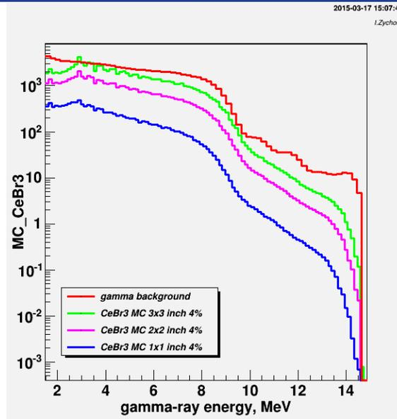
*Fig. 1. A comparison of Monte Carlo simulated detector response for CeBr<sub>3</sub> scintillators for the 0-approx. gamma-ray background used as input.*
