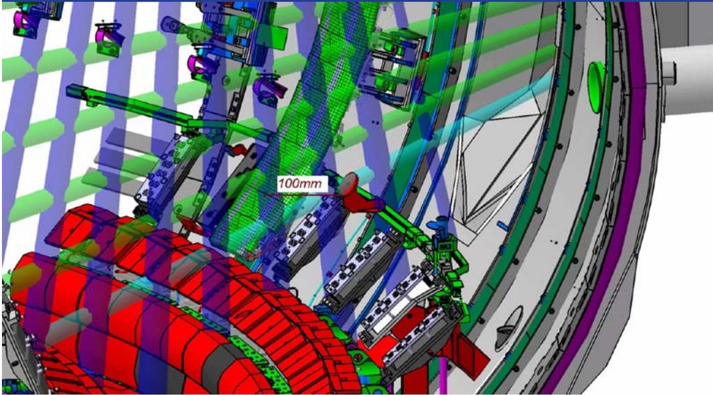
Figure 2 Distance from the limiter apex to target edge less that 100mm possible
