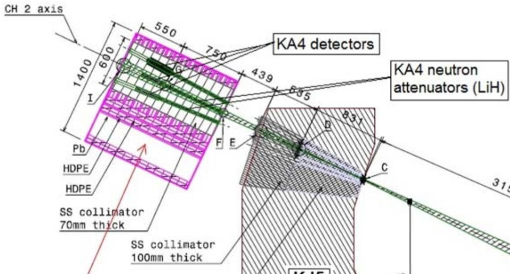
Figure 5.2: KA4 radiation collimator and shield showing also the KA4 detectors and the KA4 neutron attenuators in channels #2 and 3.
