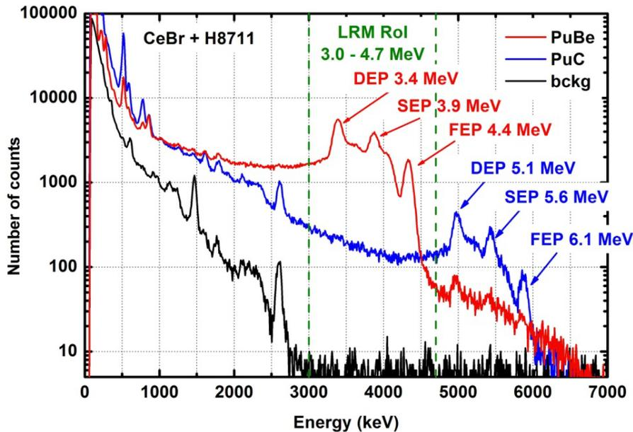
Figure 6.1: Response of a CeBr<sub>3</sub> scintillator tested at IPPLM/NCBJ
