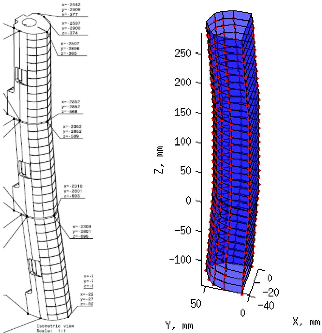
Fig.7. Drawing of the Be TAE antenna protection tile (left) and the numerical model of the tile (right) with the starting points of test trajectories marked again in red.
