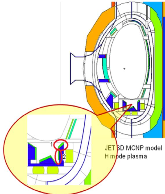
Figure 8.7: Location and numbering of the divertor cells for neutron flux and gamma production rate calculations
