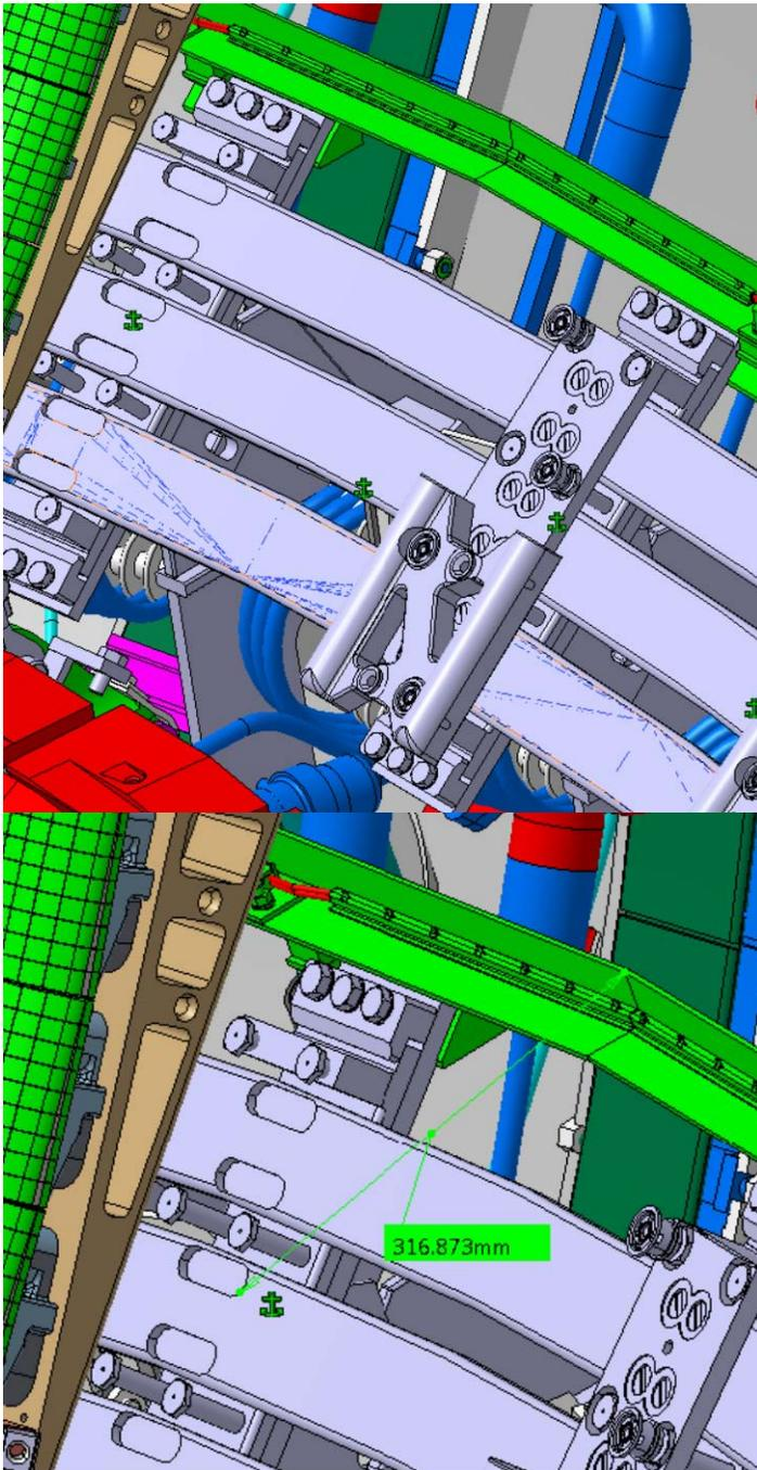
Figure 5 Sector 1C showing lower outer saddle coils where probe may be supported.
