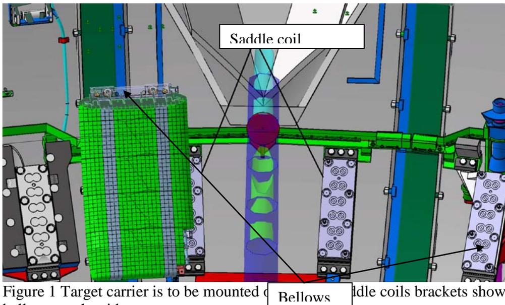
Figure 1 Target carrier is to be mounted on saddle coils brackets shown above; bellows on the sides
