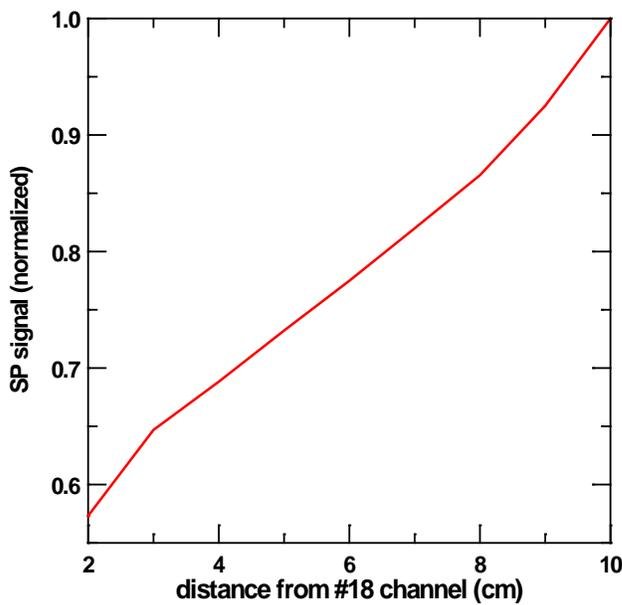
Figure 8.3: Dependence of the relative signal intensity when the LAM target moves over 10 cm away from the channel #18 LoS
