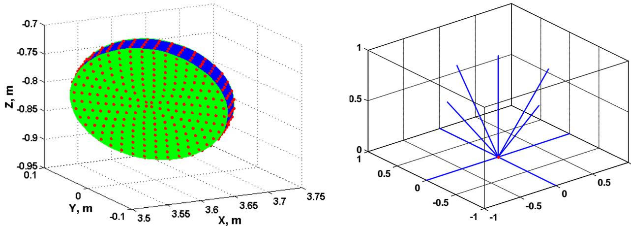
Fig.3. Left: Pellet-like LRM target with the starting points of test trajectories marked in red. Right: Starting unit velocity vectors for each starting point.
