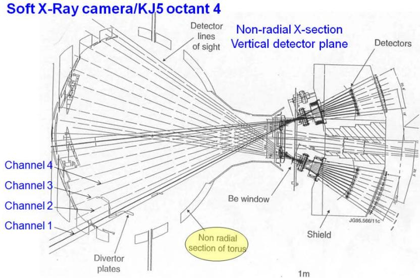
Figure 3.4: KJ5 upper soft X-ray camera (non-radial cross-section)
