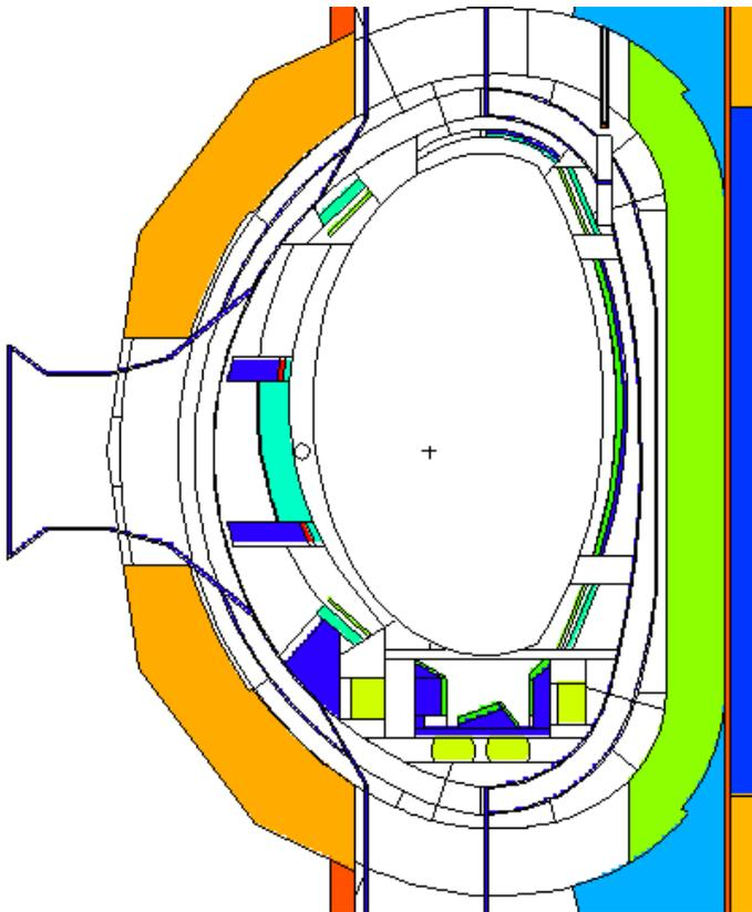
Fig. 1: Used model, 3D MCNP model of JET, H mode plasma
