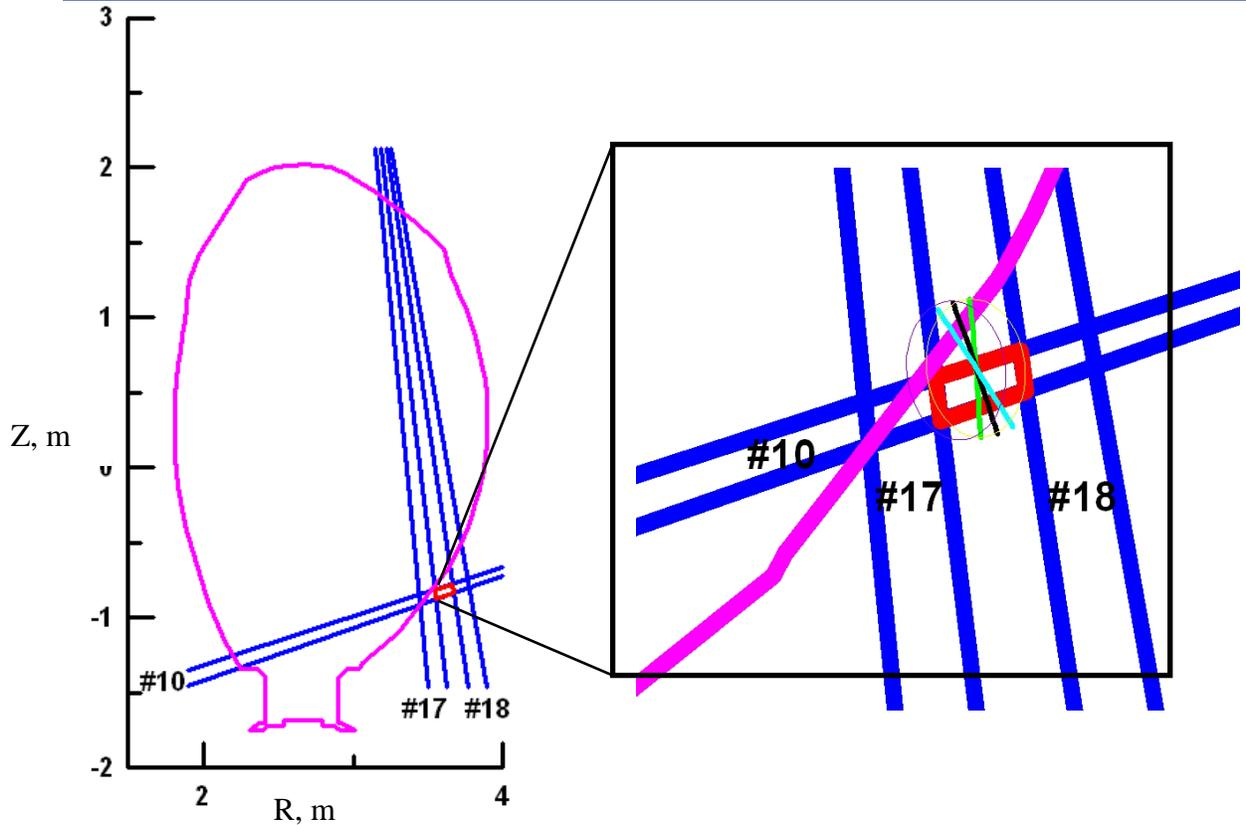
Fig.1. Expected LRM target position. Blue: gamma channels LOS. Red: possible Field of View (FOV) origin of gamma signal from LRM target. Black, green, light green: different LRM target orientations.
