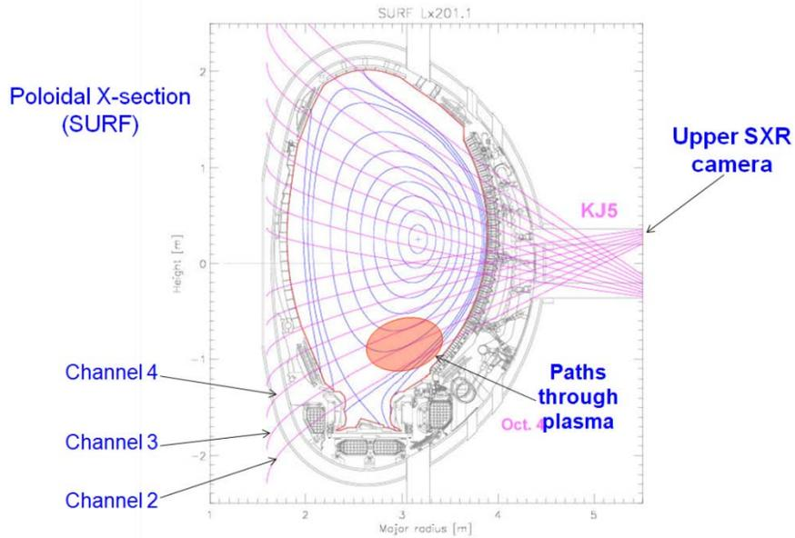
Figure 3.5: KJ5 upper soft X-ray camera with magnetic surfaces
