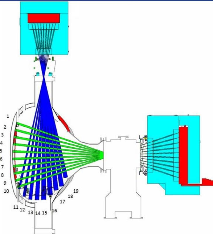
Figure 3.1: JET KN3 gamma-ray cameras showing the horizontal (1 to 10) and vertical (11 to 19) channels
