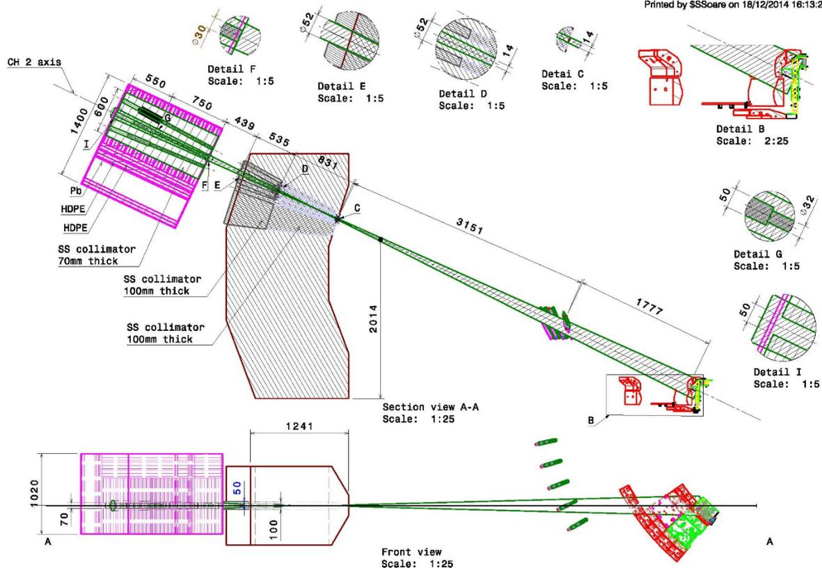
Fig. 3: The line of sight and cross-sections of the collimators with dimensions.
