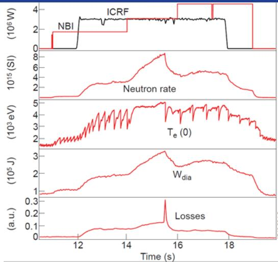
Figure 4.7: Particle losses in a JET discharge with a monster sawtooth
