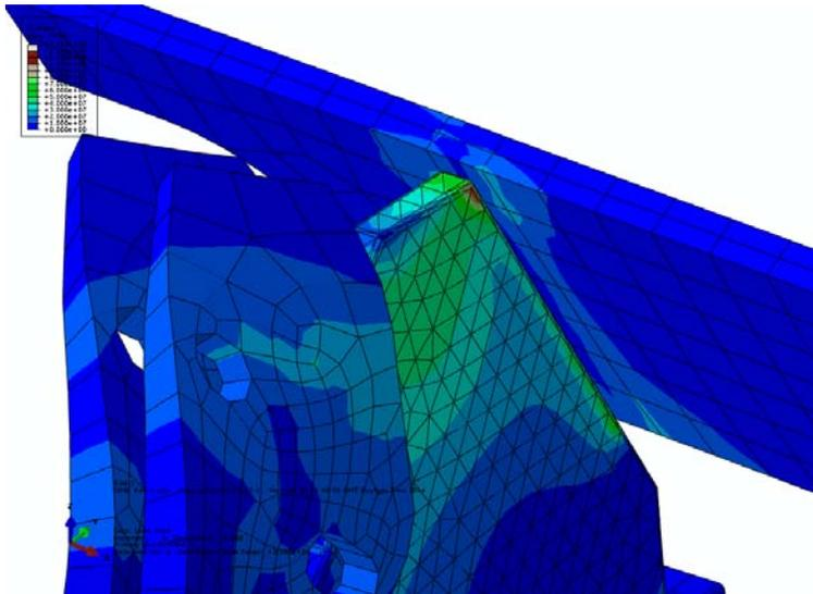
Figure 8 Close up showing that the only region is with high stress (>250 MPa) is very localised at a welded joint. FE Ref: KA4-1b
