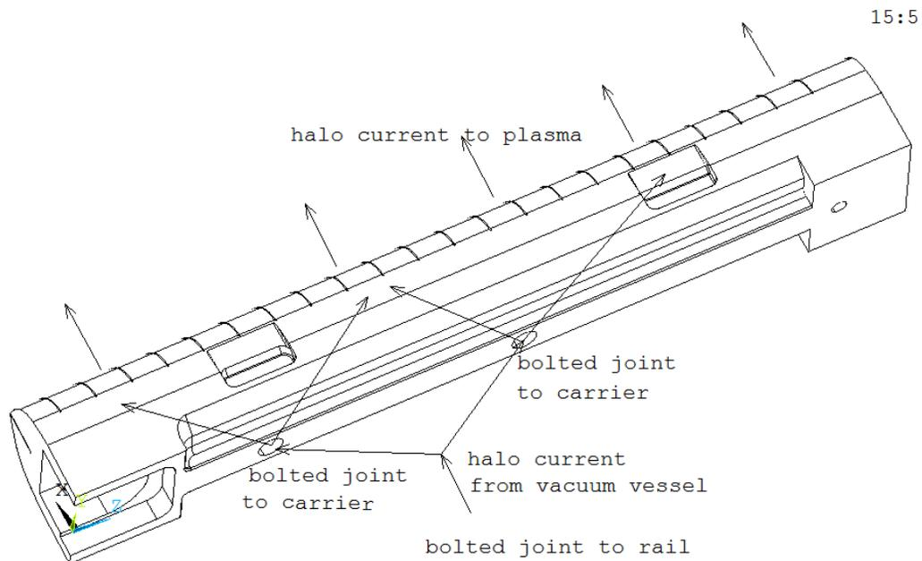
Figure 3 – Schematics on the halo current flow from the vacuum vessel back to the plasma.
