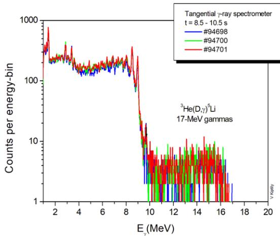
Fig. C-2 - Spectrum showing a clear evidence for the recording of  $D-^3\text{He}$  fusion gamma-rays
