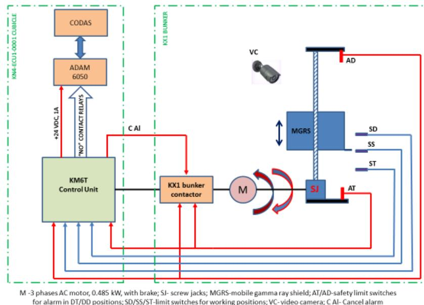
Fig. A-4 Movable Gamma-Ray Shield (MGRS) command and control. PLC: Programmable Logic Controller; Eth: Ethernet connection; CODAS: Control and Data Acquisition System
