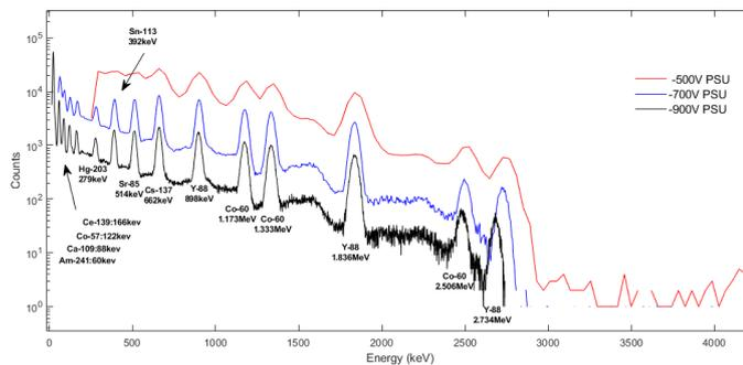
Fig. B2-4: Spectra registered when using calibration sources
