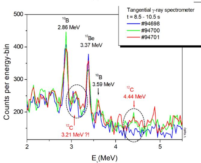
Figure B.2-1: gamma-ray spectrum from the KM6T horizontal gamma-ray spectrometer developed by the GSU project and measured in JET discharges #94698, 94700 and 94701 from the 3 ion ICRH experiment M18-11.
