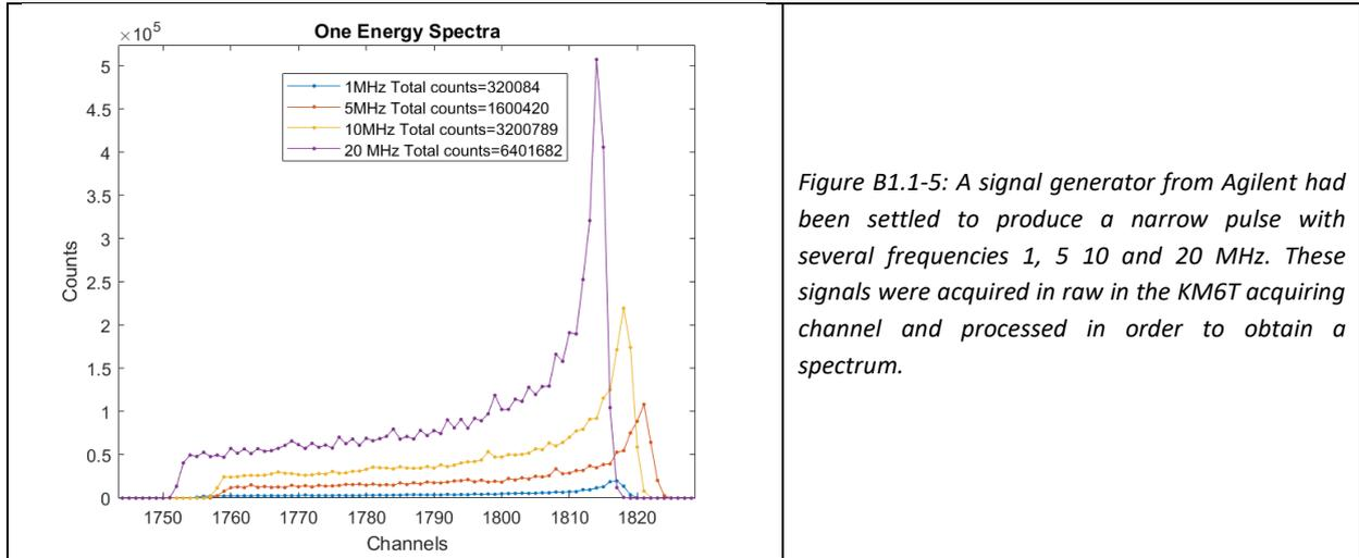
Figure B1.1-5: A signal generator from Agilent had been settled to produce a narrow pulse with several frequencies 1, 5 10 and 20 MHz. These signals were acquired in raw in the KM6T acquiring channel and processed in order to obtain a spectrum.
