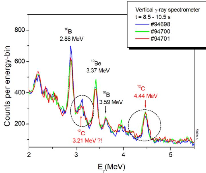
Figure B.2-2: gamma-ray spectrum from the KM6S vertical gamma-ray spectrometer measured in JET discharges #94698, 94700 and 94701 from the 3 ion ICRH experiment M18-11.
