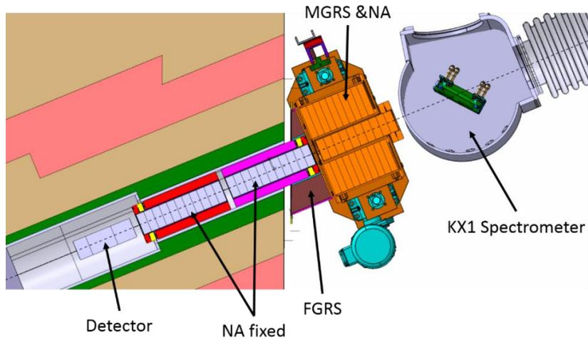
Fig. A-2 Radiation Field Components Assembly at the detector end of the KM6T beam-line. MGRS: Movable Gamma-Ray Shield; FGRS: Fixed Gamma-Ray Shield; NA: Neutron Attenuator
