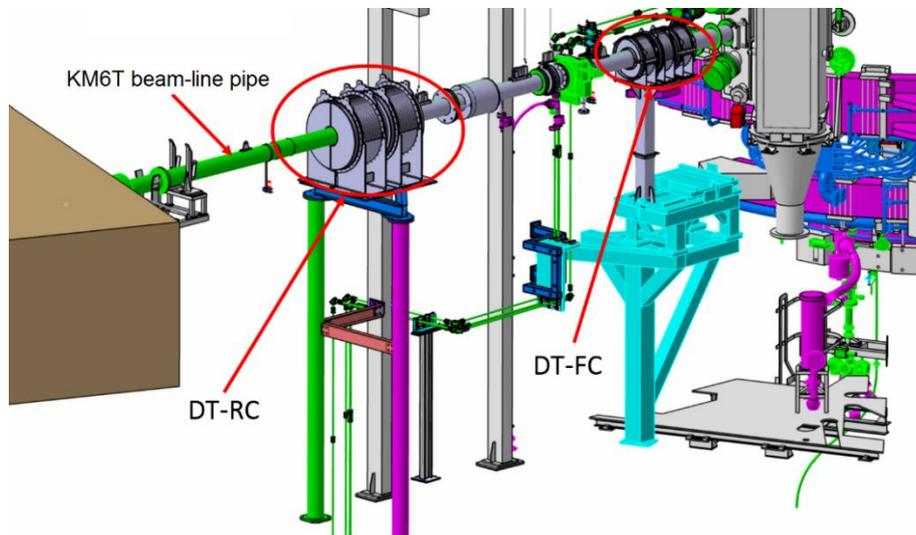
Fig. A-1. Upgraded KM6T tandem collimators. DT-FC: Front Collimator for DT pulses. DT-RC: Rear Collimator for DT pulses.
