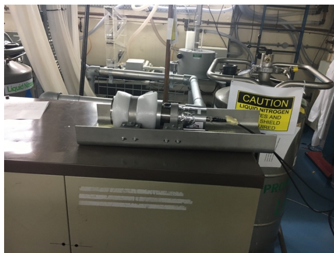
Fig. 2. Stand for measurements at JET lab with radioactive sources: ^{137}\text{Cs} , ^{60}\text{Co} and ^{22}\text{Na} .
